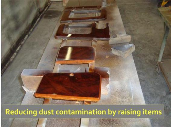
thinners onto the finish. The tin of thinners may need to be changed a number of times during the finishing process. If the paint brush becomes contaminated with dust & other particles, it should be washed in water and detergent.
