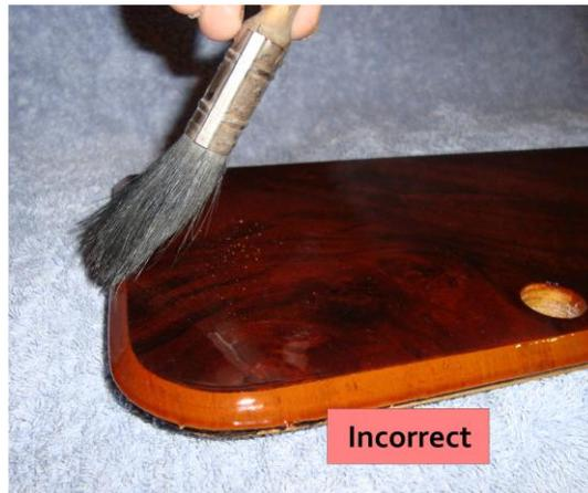
If the job has been under-stained, a small amount of stain can be added to most clear finishes. Always mix a small test batch to evaluate compatibility and depth of colour. It should be applied after the second coat. Mix up a separate batch so you can go back to the un-coloured finish for the final coats. Apply another 3 clear coats before you start sanding back.
