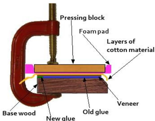
Alternately use a scalpel to scrape old glue from the gap formed by the lifted veneer. Work 5-minute-Araldite into the gap with a scalpel. If a slower drying time is required, use high strength Araldite. PVA wood glue is not recommended. Clamp as follows: Lay several layers of cotton cloth over the repair, followed by a foam pad, then a block of wood. Clamp together with a 'G' clamp; not too much pressure.
